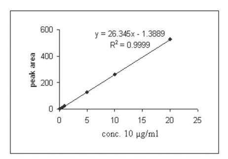
Figure 2. Calibration curve of standard hydroquinone solutions
