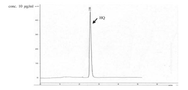
Figure 3. HPLC chromatogram of standard hydroquinone solution (conc. 10 µg/ml)
