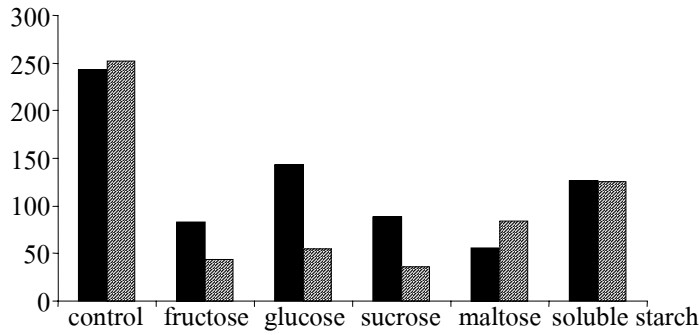
Fig. 2 Effect of carbon source on production of the enzyme (■) 0.5% carbon source, (▨) 1.0% carbon source.
