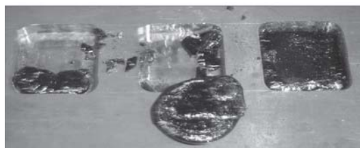
Figure 1. The ceramic samples with nominal compositions of \text{Bi}_2\text{Sr}_2\text{Ca}_2\text{Cu}_3\text{O}_{10} were melt-quenched method at 1200^\circ\text{C} for 30 min.
