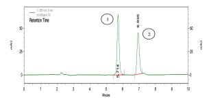
Figure 3. The chromatogram of two standard capsaicinoids (peak 1 : capsaicin and peak 2:dihydrocapsaicin)
