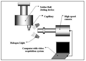
Figure 4. Schematic drawing of experiment setup.
