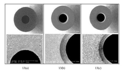
**Figure 13**. 13a) Capillary type A: Conventional capillary, 13b) Capillary type B: Chamfer edge capillary, 13c) Capillary type C: Fillet edge capillary
