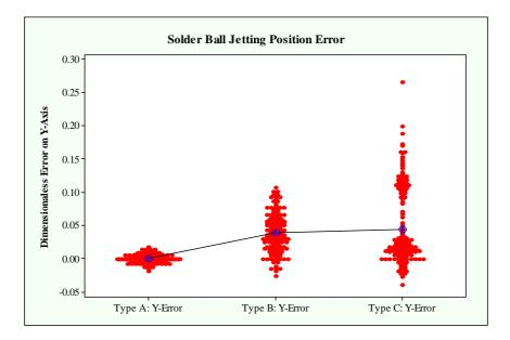
Figure 10. Comparison of solder ball jetting position error in Y-direction
