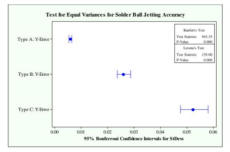
Figure 12. One-way ANOVA testing of solder ball- jetting accuracy in Y-direction
