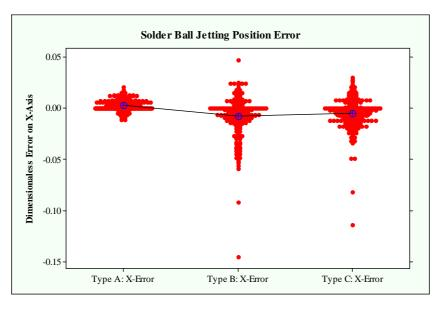
Figure 9. Comparison of solder ball jetting position error in X-direction.
