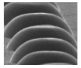
**Figure 15.** Solder joint surface performed by capillary type A.
