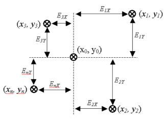
Figure 3. Solder ball jetting accuracy schematics in laser solder ball jetting process.
