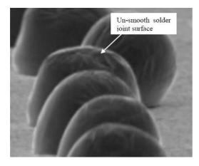
**Figure 16.** Solder joint surface performed by capillary type B
