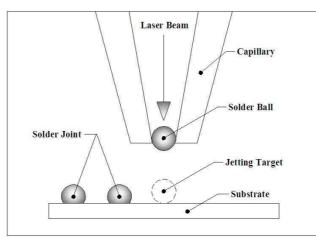
Figure 1. A solder ball was hold by capillary tip and laser energy applied to melt the solder ball.
