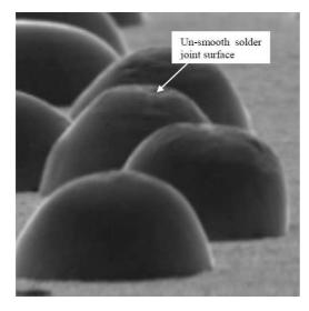
**Figure 17.** Solder joint surface performed by capillary type B
