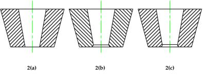
Figure 2. (a) Capillary type A, (b) Capillary type B, (c) Capillary type C.
