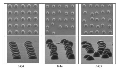
**Figure 14.** Solder joint array, 14a) Perform by capillary type A, 14b) Perform by capillary type B, 14c) Perform by capillary type C.
