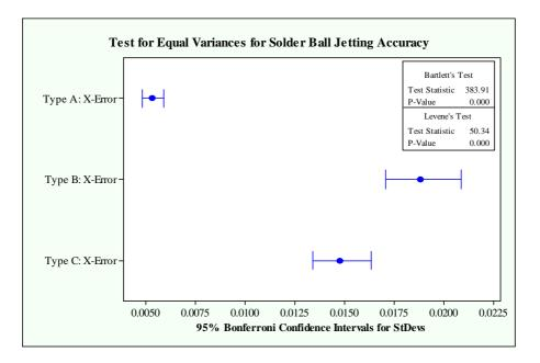
Figure 11. One-way ANOVA testing of solder ball-jetting accuracy in X-direction
