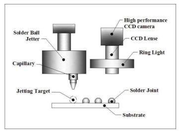
Figure 5. Schematics plot of Solder Ball Jetting Accuracy testing.
