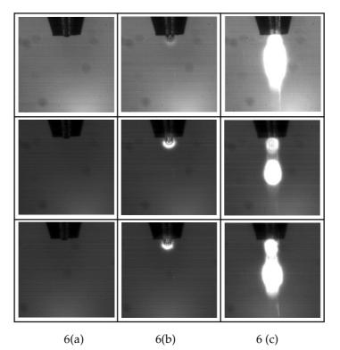
**Figure 6.** Solder ball jetting process. 6a) The capillary with solder ball before laser apply; solder ball is dark. 6b) The solder ball start to move out from capillary after laser energy applied; color changing in solder ball. 6c) Completely melt solder ball jetting from capillary.
