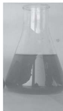
Figure 6. Photograph of effluent color from hybrid system at 203 SU
