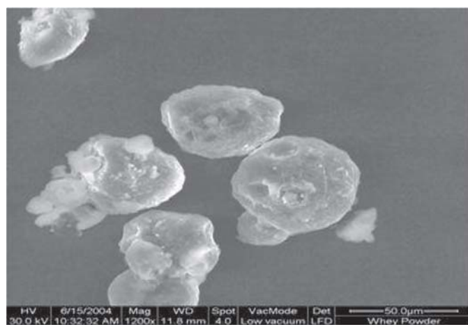
Figure 2. SEM image of whey powder at high resolution showing the loose aggregation of the primary whey particles (Magnification = x1200)
