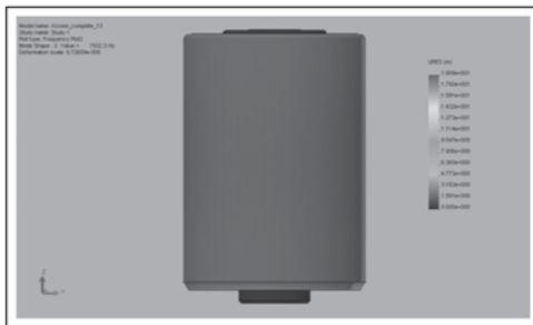
Figure 12. The mode two of the bearing simulation at frequency of 7932.3 Hz.
