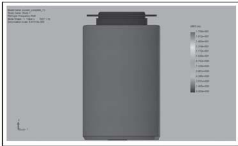
Figure 11. The mode one of the bearing simulation at frequency of 7657.1 Hz.
