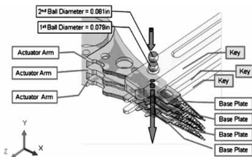
**Figure 1.** Prototype of the ball swaging process
