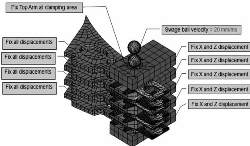
**Figure 2.** Display the define boundary condition for the finite element method with the normal ball direction.
