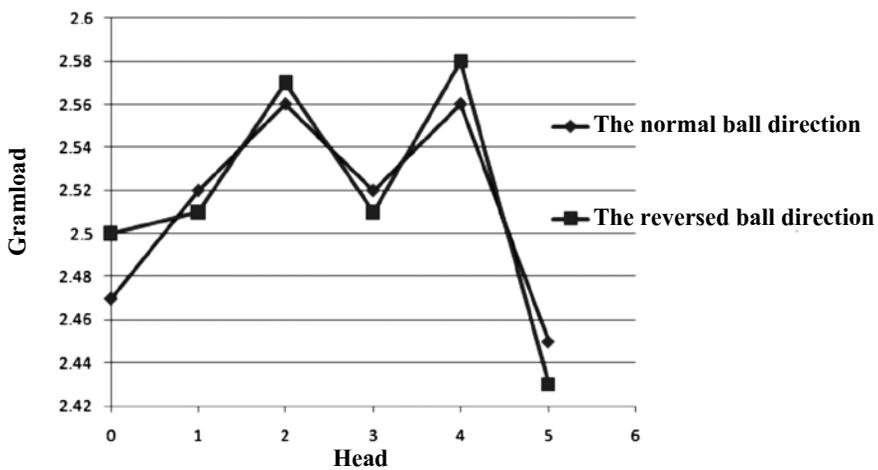
**Figure 9.** The comparison of the gram load from the analysis using the finite element method between the normal ball direction and the reversed ball direction.
