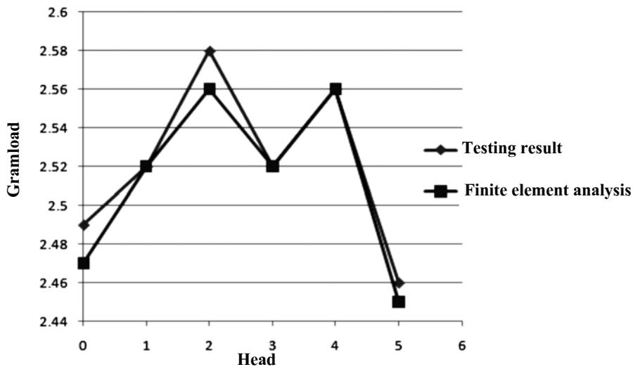
**Figure 7.** The graph showed the comparison of the gram load from the normal ball direction between finite element method and the ball swaging process.
