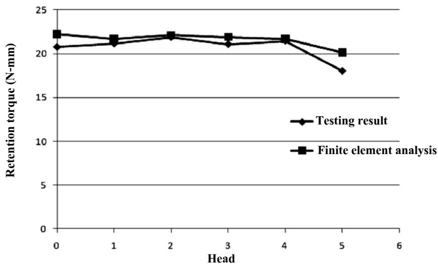
**Figure 6.** The graph compared the average retention torque between the finite element method and the ball swaging process with the normal ball direction.
