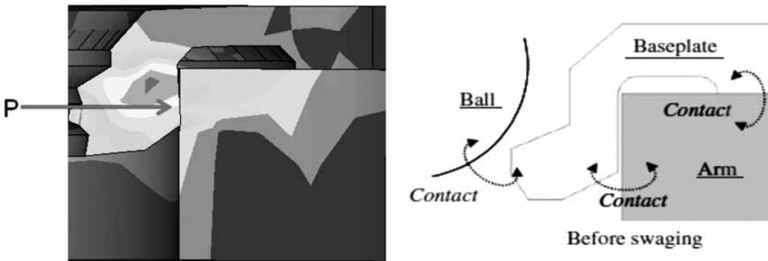
**Figure 4.** Shown the contact pressure of the surface generated to the actuator arm
