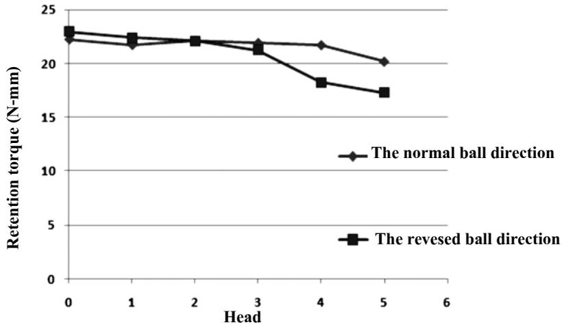
**Figure 8.** The comparison of the retention torque from the analysis using the finite element method between the normal ball direction and the reversed ball direction.
