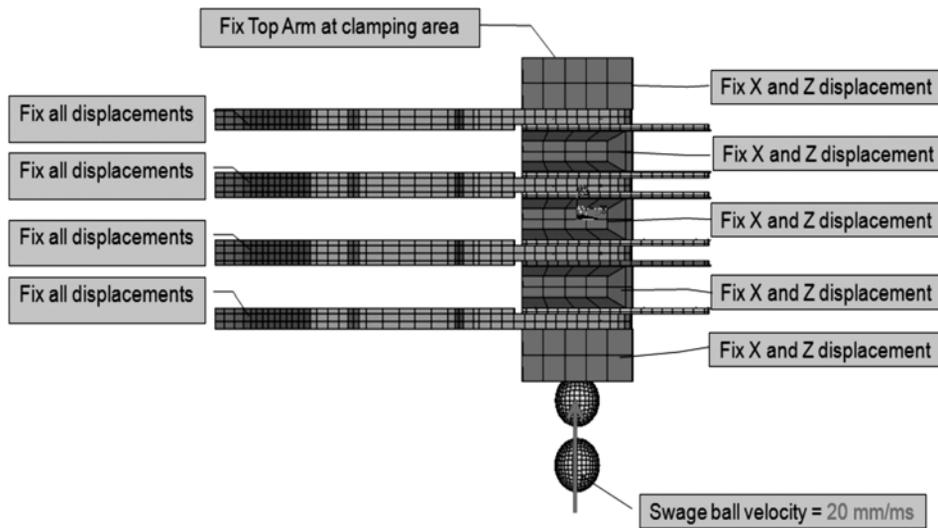
**Figure 3.** Display the define boundary condition for the finite element method with the reversed ball direction.
