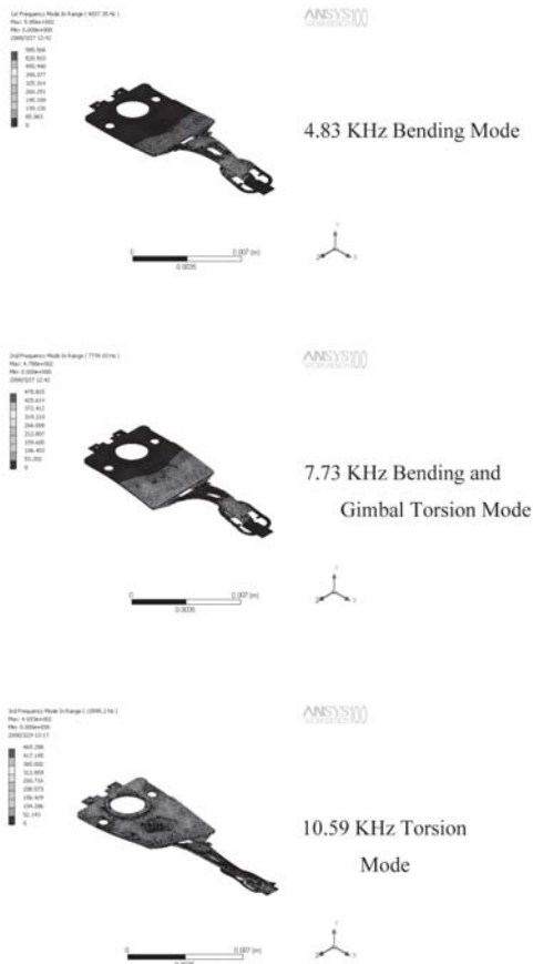
Figure 4. Mode shape of HGA vibration from simulation
