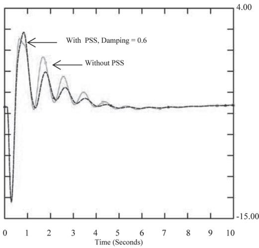
Figure 13. Rotor angle time domain with PSS at designed damping 0.6
