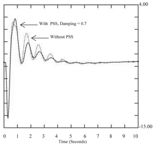
Figure 14. Rotor angle time domain with PSS at designed damping 0.7
