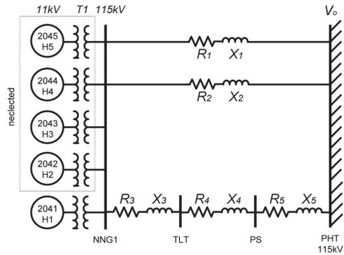
Figure 5. Single line diagram of Nam Ngum 1 H/P connected to the infinite bus at Phonetong S/S.
