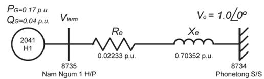
Figure 6. Equivalent system of single machine connected to a large system through a transmission line.
