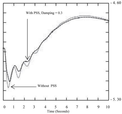
Figure 8. Rotor angle time domain with PSS at designed damping 0.3
