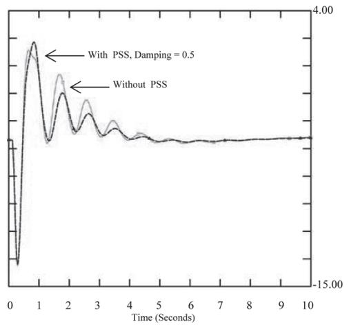
Figure 12. Rotor angle time domain with PSS at designed damping 0.5
