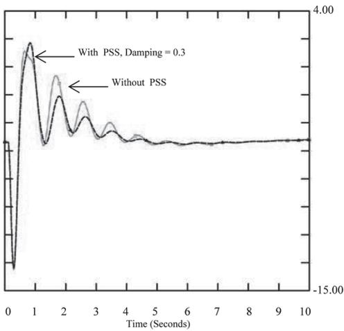
Figure 9. Rotor angle time domain with PSS at designed damping 0.3
