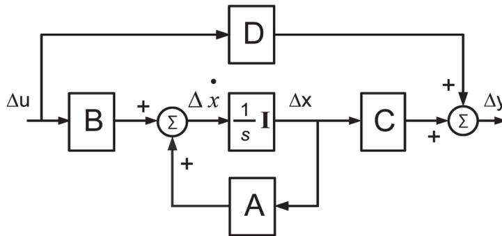
Figure. 3 Block diagram of the state-space representation
