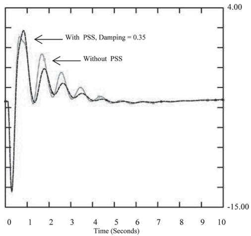
Figure 10. Rotor angle time domain with PSS at designed damping 0.35
