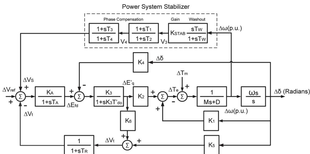
Figure 4. Small perturbation transfer function block diagram of a single machine-infinite bus associated with conventional PSS
