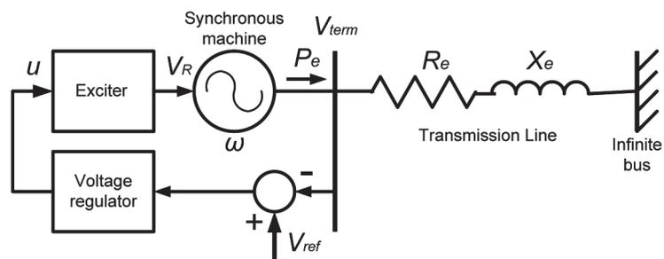
Figure 2. Single machine-infinite bus system
