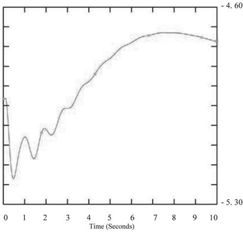
Figure 7. Rotor angle time domain without PSS from pervious study
