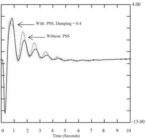
Figure 11. Rotor angle time domain with PSS at designed damping 0.4
