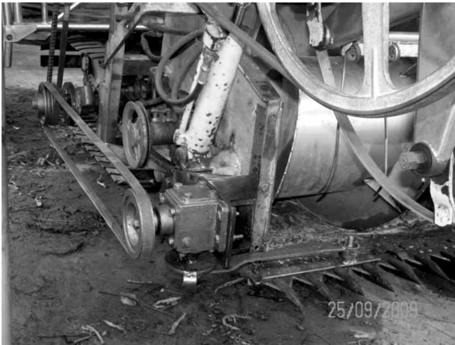
Figure 5. Cutter Bar Driver (Perpendicular Axle, Driven by Chain)
