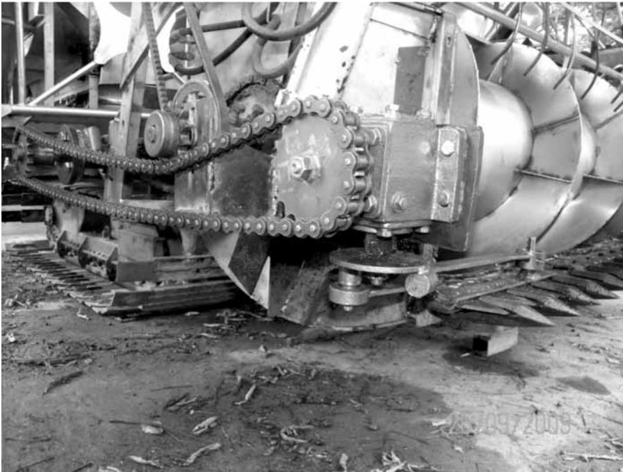
Figure 4. Cutter Bar Driver (Perpendicular Axle, Driven by Chain)
