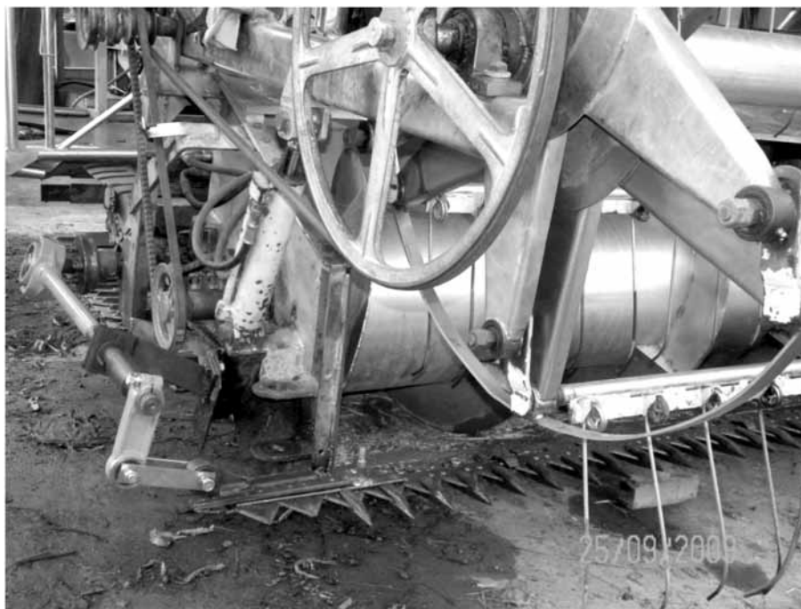
Figure 3. Cutter Bar Driver (Stir Type)
