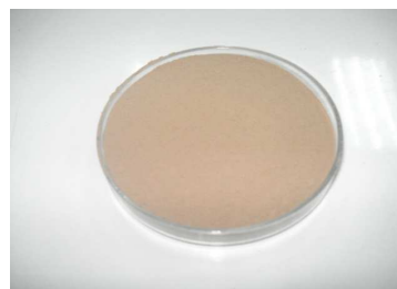
Figure 1. Alum sludge after grinding through a No. 100 sieve.
